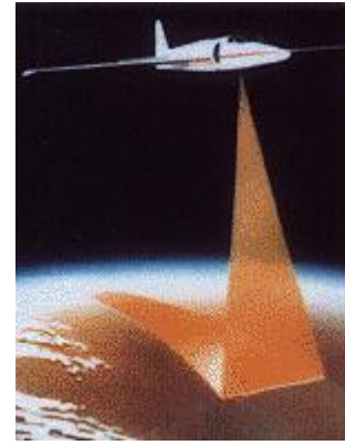
Figure 9 – HSI sensors capture data one line at a time, forming an image cube from many adjacent lines as the sensor moves forward [17]
