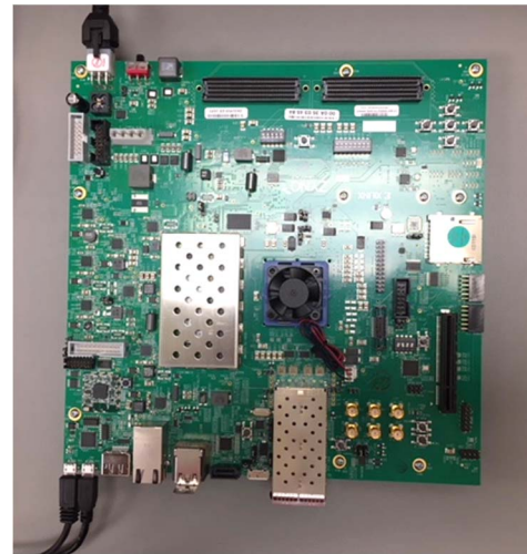
Fig. 2. ZU9EG DUT (under heatsink) on ZCU102 evaluation test board.
