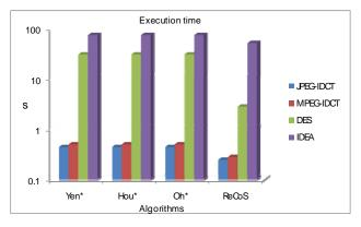
**Figure 2**: ReCoS algorithm execution time compared against enhanced reconfigurable aware Yen, Hou, and Oh algorithms on 1M blocks of data.
