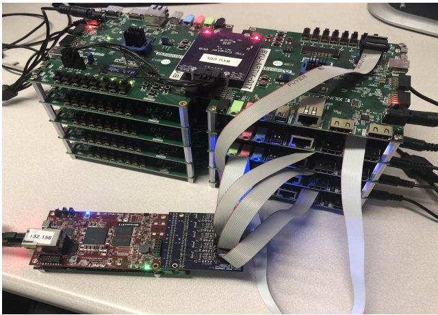
Fig. 3. Multiple TURTLE FI platform featuring two XC7A200T devices per layer.
