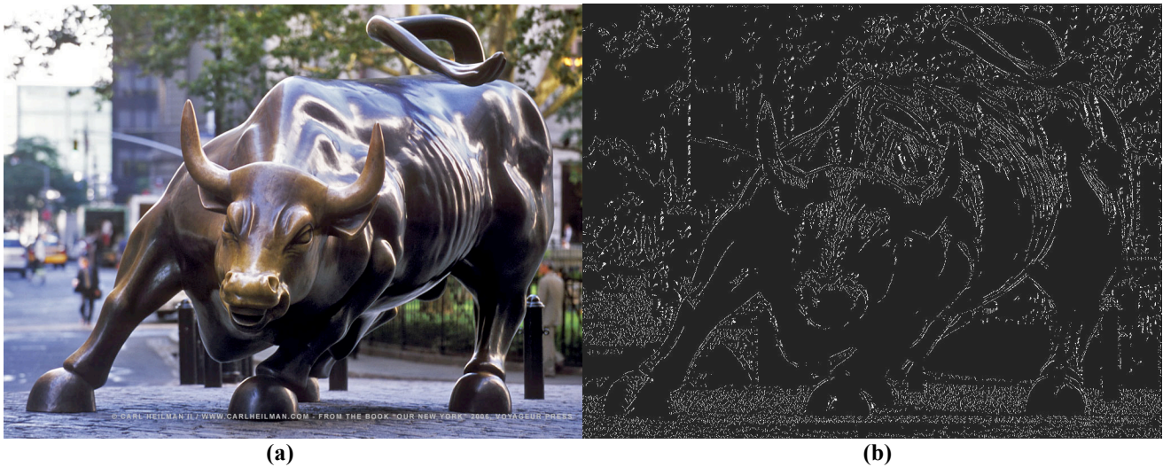
Figure 3: a) The original Wall Street bull image used for Canny filter processing. b) The output image after Canny filter processing.
